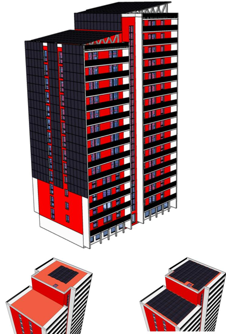
*The high-rise building form tested with integrated façade and monopitch PV panel design. SAP baseline and concertina maximum roof mounted outputs were also calculated, considering perimeter access corridors for both layouts.*
