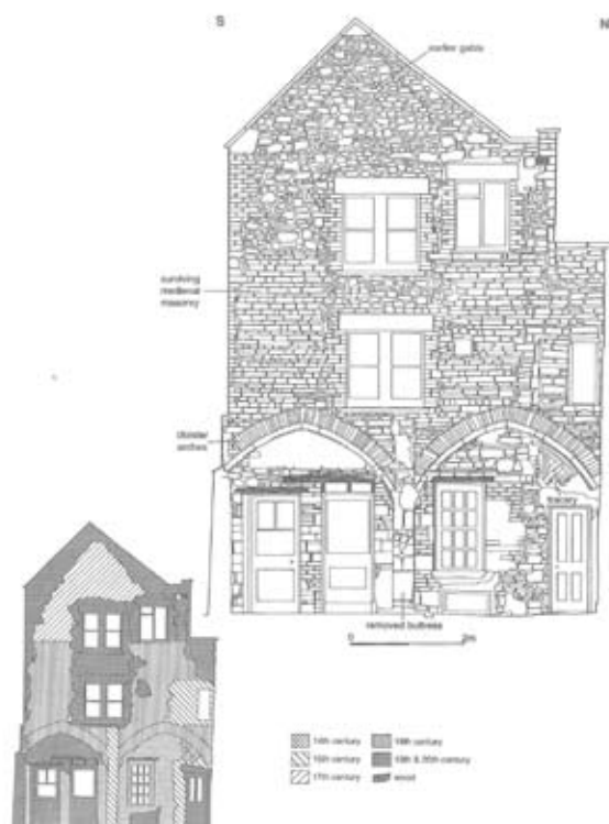
Figure 17: A survey of the exterior of the rear wall of Church House showing the arches and tracery of the west range of the cloisters
