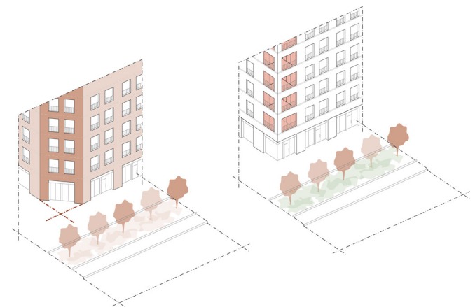
Diagram 16 - Chamfers and nooks can increase visibility, whilst corner balconies can overlook and animate the public realm.
