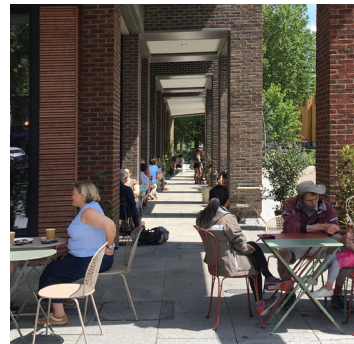
Image 22 – Colonnades can provide shelter and shade, as well as threshold for spill out activity from ground floor units. © Panter Hudspith.
