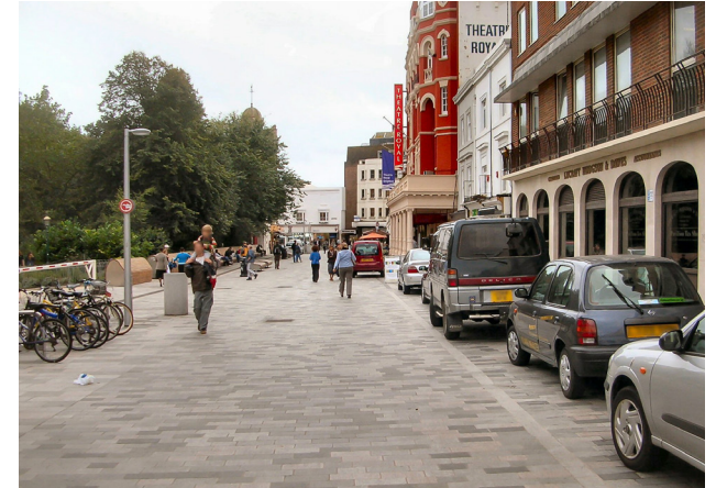
Image 16 – Vehicles servicing areas denoted through a subtle but clear change in material. © DeFacto, CC BY-SA 2.5 , via Wikimedia Commons
