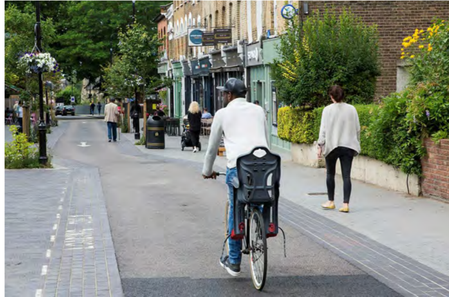
Precedent: Orford Road, Walthamstow. The one way movements allow for the carriageway to be reduced to allow for footways to be widened while allowing contra-flow cycling. New street trees have also been planted.
