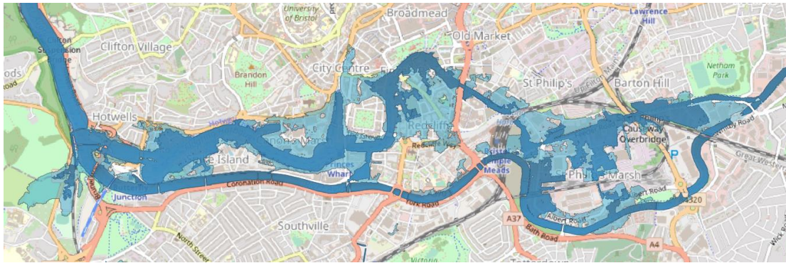
Figure 1: Do Nothing 1 in 2 annual chance tidal flood outline, 2045 (dark blue) and 2125 (light blue).
