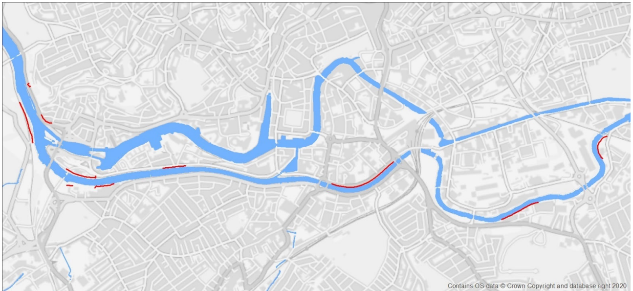
Figure 20: Sections of Phase 1 flood defence in Bristol that are raised to prevent detriment in 2130.
