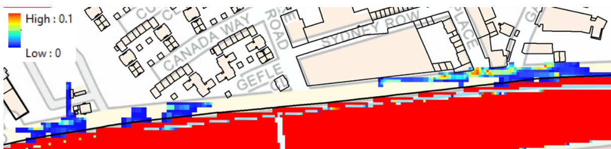
Figure 25: Flood depths for 1:200yr tidal event in 2130 for 200yr SoP scheme model.
