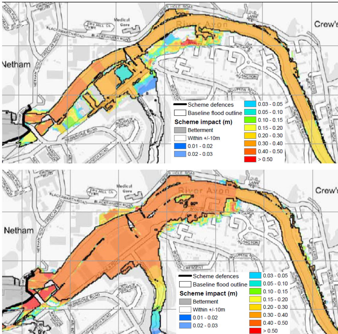
Figure 22: Example of detriment from SOC defences without detriment mitigation, fluvial 1:100yr event in 2065 (top) and 2130 (bottom).
