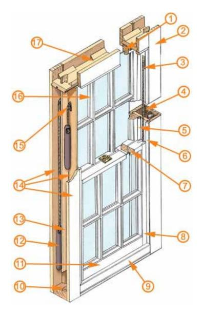
1 Top Rail - the top horizontal framing member of a sash
