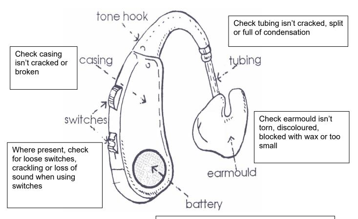
Check battery compartment for signs of corrosion. Check battery is working by listening for feedback (whistling sound) when the hearing aid is switched on and covered in a cupped hand.
