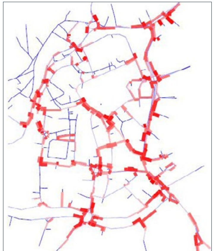
Fig 8: PARAMICS Microsimulation Model Output, Bristol City Centre
