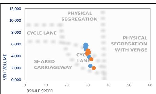
The diagram compares total daily traffic flow (vertical axis) against the average daily 85%ile speed (horizontal axis) to demonstrate cyclist and vulnerable user considerations.
