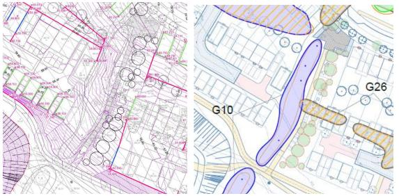
The only section of hedgerow proposed for retention G10 has significant earthworks on either side which is likely to lead to the loss of this feature.
