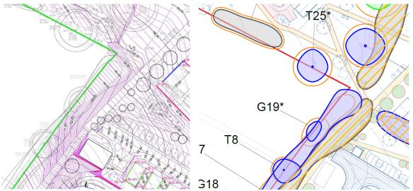
The addition of up to 3m of material to facilitate a footpath on north-western boundary of the site adjacent to the allotments and within the root protection areas of T8 & G19 (Which includes Holly T6 TPO 1404) has the potential to adversely affect the rooting environment of the trees which can lead to their decline and early loss.
