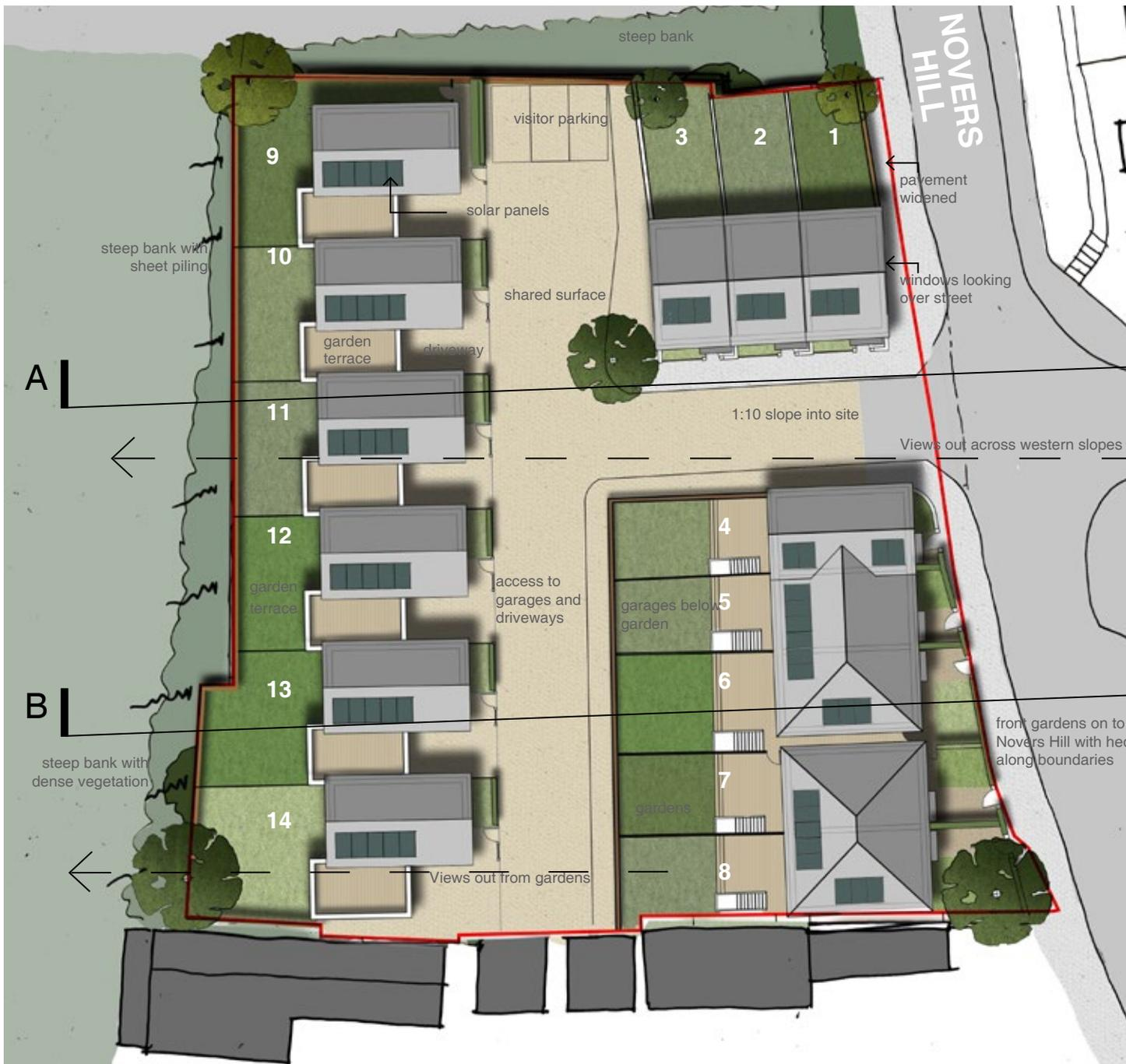
6.3 The topography of the site makes access a significant factor in the layout. In order to get vehicular access at a suitable gradient the proposal creates a central shared road serving the units overlooking the slopes to the west and also providing access to garages for the units fronting Novers Hill.
