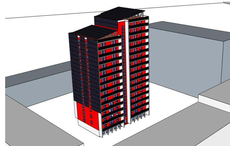
*A 3D model of the flats and surrounding features was created in DesignPH 2.0.06 and used to calculate solar gains and shading for PHPP.*
