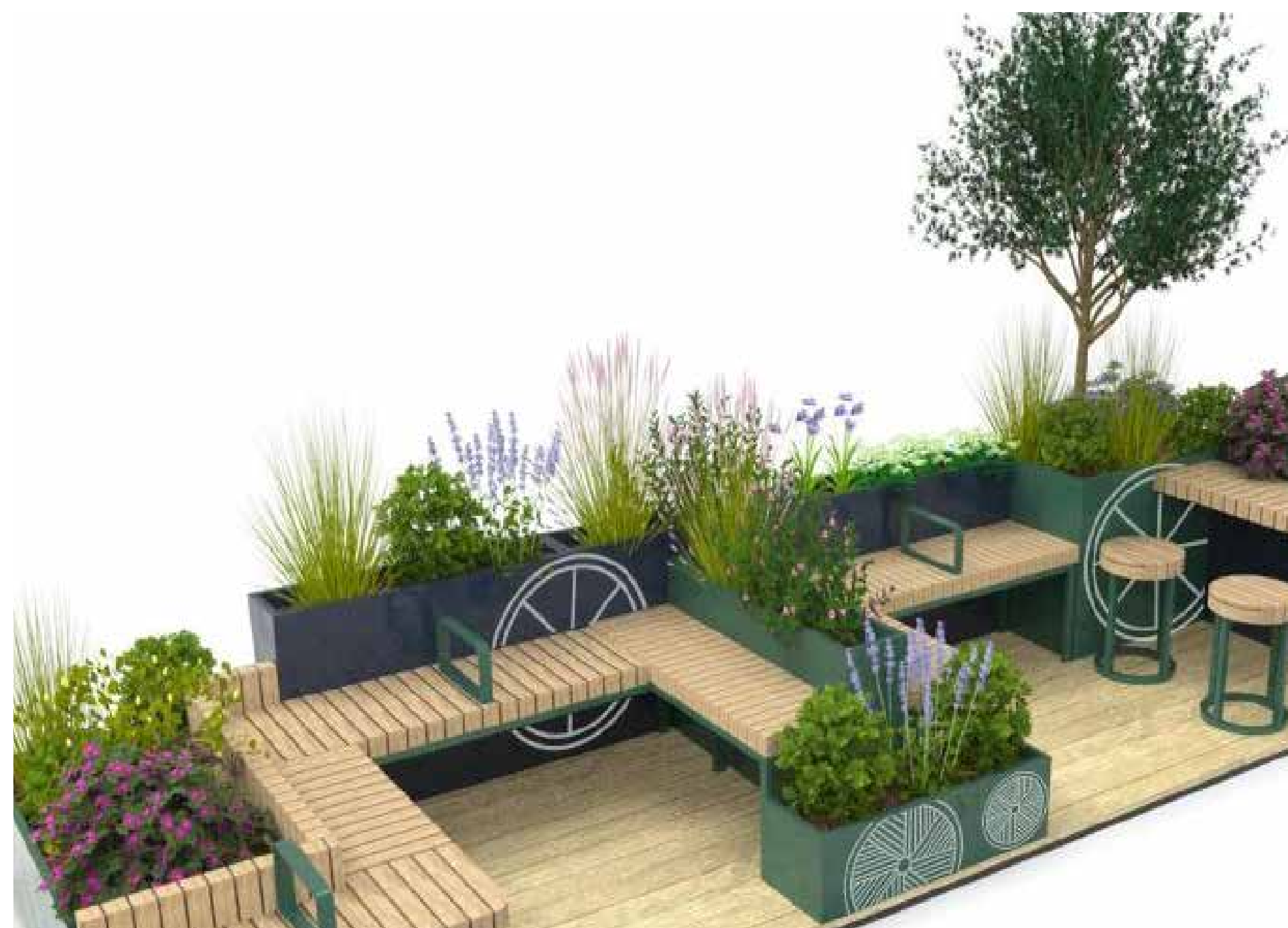
The semi-enclosed seating areas will be open on the shops side. They will be designed so that they go straight on the ground without a deck
