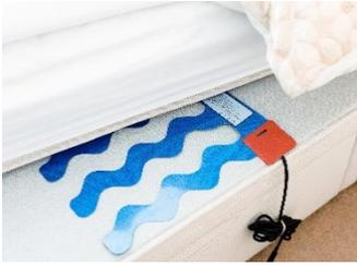
Technology enabled care (TEC) can be used to monitor individuals living with epilepsy while they sleep. Seizure activity is often complex, but epilepsy sensors can be used to help detect Tonic-Clonic seizures. They are normally placed under the mattress of the bed and used overnight. They work by detecting when combinations of continuous movements and noise differ to normal patterns and behaviours.
