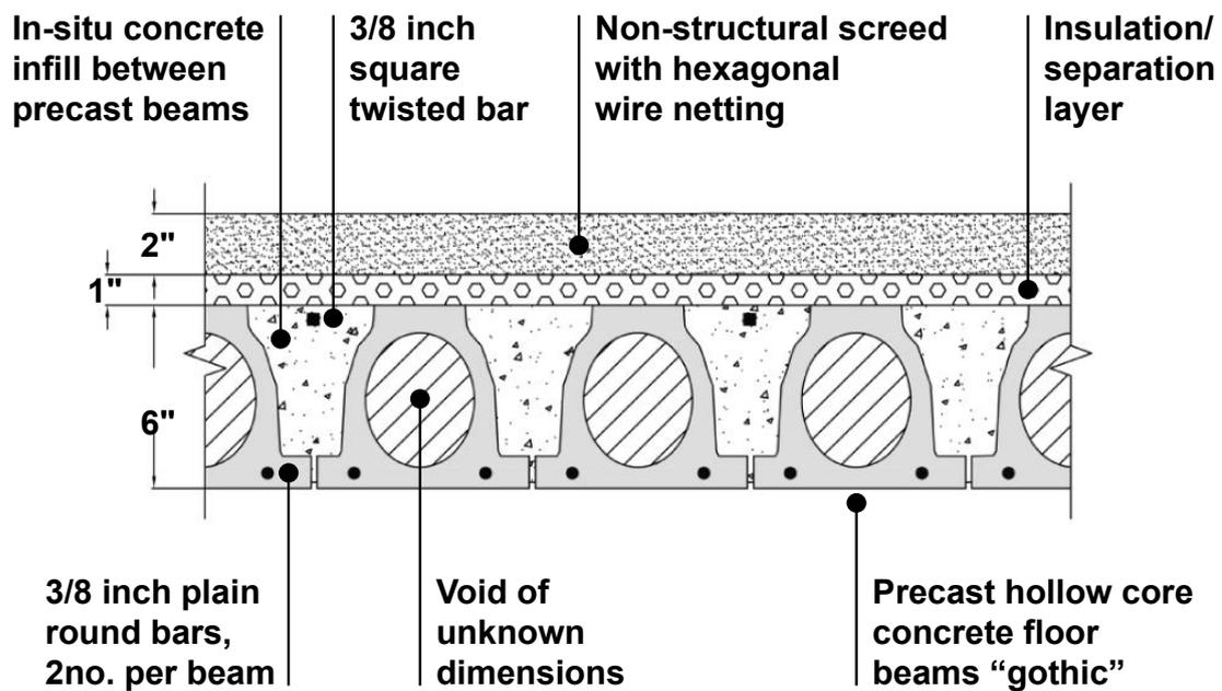
The original drawings specified 1/2" (13mm) cover to slab reinforcement. Our observations from the site survey carried out indicates that the bottom concrete cover to the reinforcement varied from 10mm -15 mm; this aligns with Ridge's reported observations their second report.
