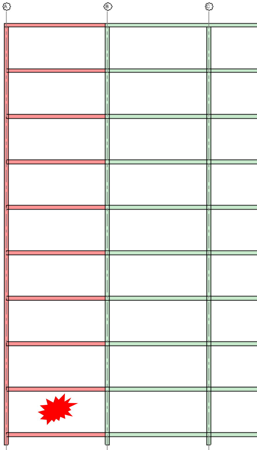
Figure 21 – Collapse mechanism if fire event occurs within a flank wall flat, Haviland & John Cozens house (elevation)
